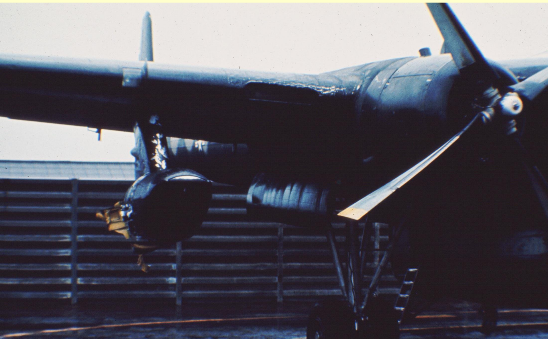
AC-119K Stinger Gunship (jet engines, FLIR, 2 ea 20 mm Vulcan Gatling Guns)
