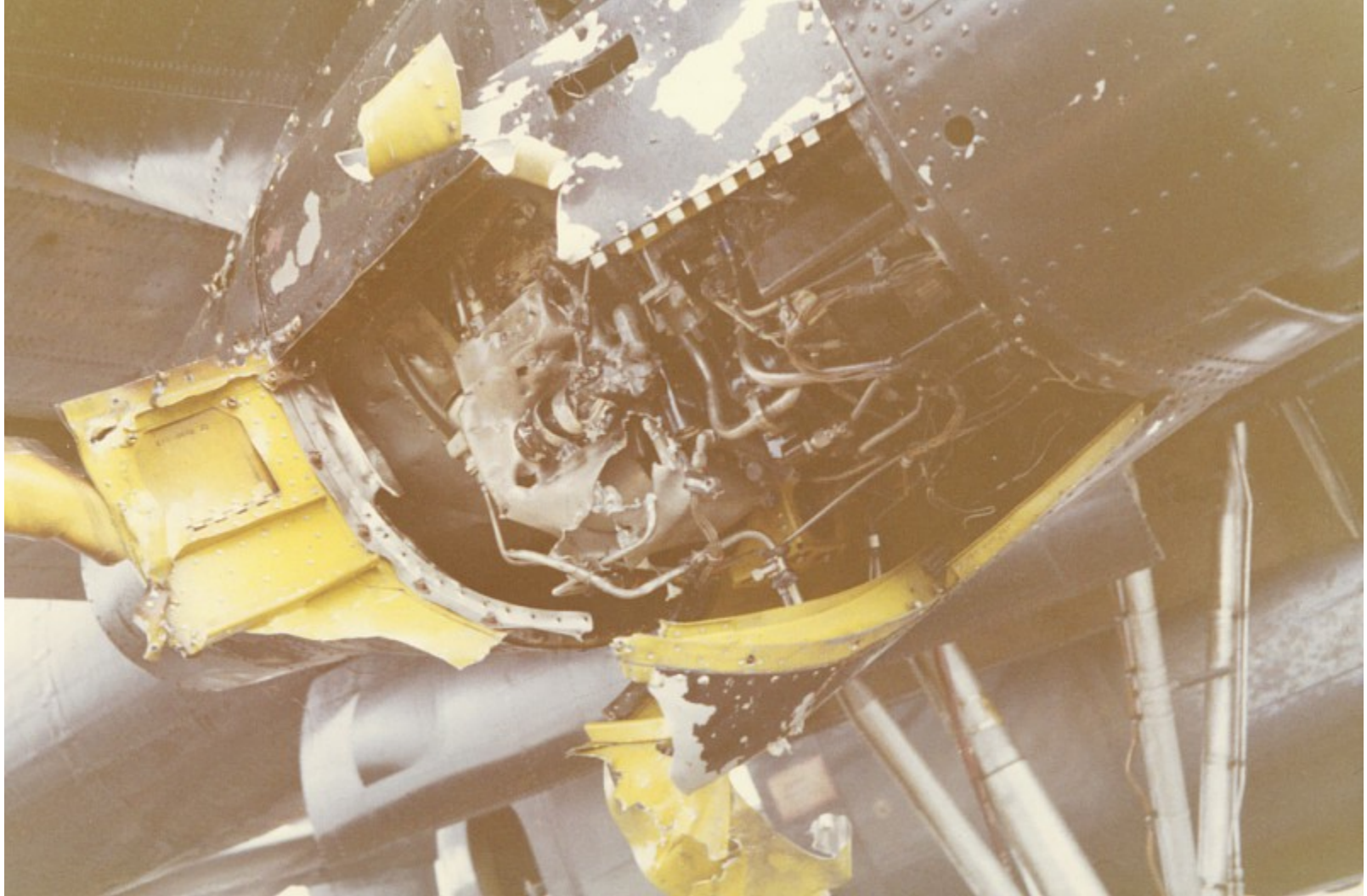
AC-119K J85 JET ENGINE WITH BATTLE DAMAGE
