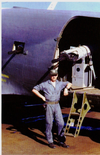
The AC-47 was armed with three 7.62mm (GAU-2/M134) Miniguns that were capable of firing up to 2,000 rounds per minute. The weapons were lethal against any convoy caught on a straight stretch of road or trail. This photo was taken at Bien Hoa in the late 1960s.
