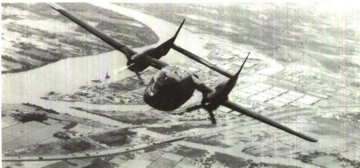
AC-119G "Shadow" Gunship in Firing ATTITUDE: Note 7.62mm Miniguns
