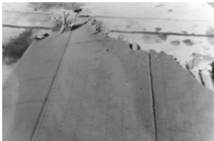
Missing 14' of Wing Tip and it Flew Back
